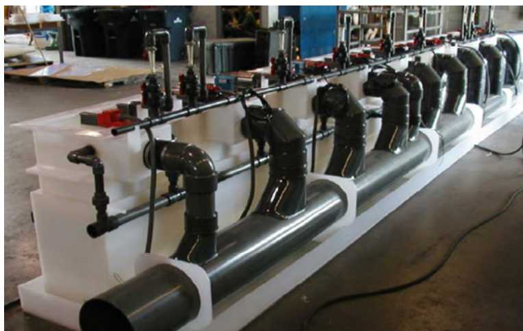
PP Process Tanks with PVC Piping
